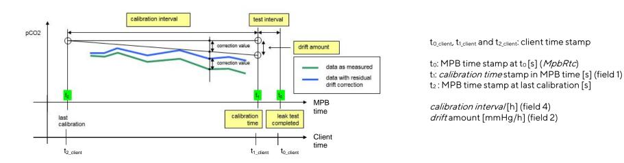
**Note:** The Sentec Digital Monitor is able to output a "Full Memory Dump" (via command: "/historical\_data/get/") where the PCO2 values as well as drift corrected PCO2 values of (a) measurement(s) are shown in columns. A validation of the calculated, drift corrected PCO2 values can be made by doing a comparison between the SDM output and the calculated values.
